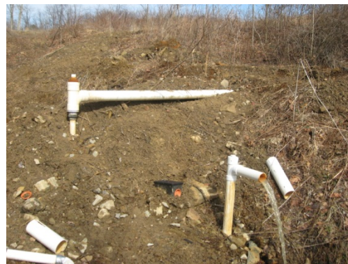
Figure 11. TROMPE in operation.
